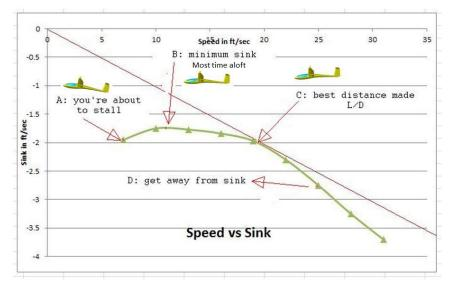
B: sink = -1.75 ft/sec so from a 500' launch height you would be on the ground in 4.76 minutes and traveled 3135 feet C: sink = -2 ft/sec so from a 500' launch height you would be on the ground in 4.2 minutes and traveled 4500 feet Hopefully the decalage angle along with setting the CG as above will result in a good cruise speed – see C: in the graph.
