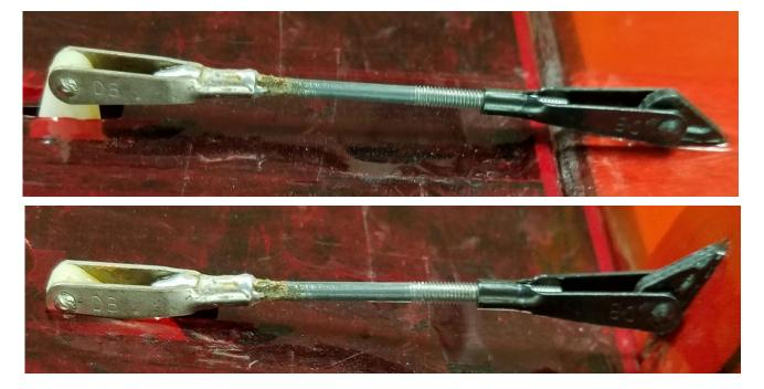
Servo arms neutral position should be at right angles to the push rod. Mount rudder and elevator servos out of the way under the wing if possible. This will leave more room up front for receiver, ESC, and battery placement and balancing flexibility.
