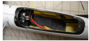
I recommend that with a sailplane you start testing with the CG at 38% Of the MAC (mean aerodynamic chord). (flying wings start at 15% - power planes start at 25%)
