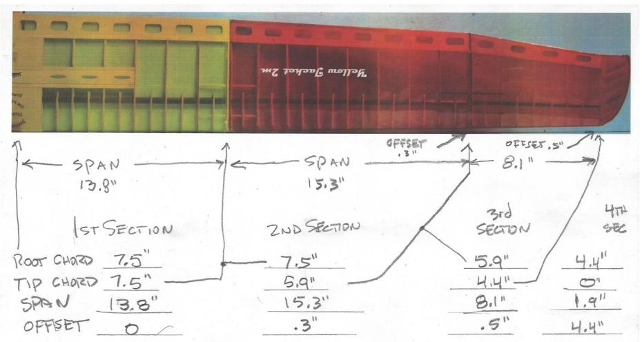
Determining MAC – I have a program on an Excel spreadsheet. Just need these measurements.
